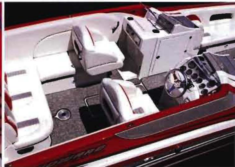
Left: Howard installed an IMCO Marine tilt helm and a full complement of Livorsi Marine gauges at the driver's station. Right: Covered with snap-in carpet, the cockpit of the 28 Sport Deck featured twin bucket seats and an L-shape bench.
